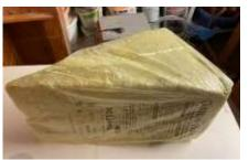
4 triangular cuts fit in one bin-liner. Both packs of Rock-Wool (6 plates each) result in 24 triangular packs. That is enough for a room height of 2.4 m. I built the absorbers only about 1.9m high and therefore got by with 18 packs.
